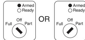
2. **Either** turn the keyswitch to "Full" to set Level A **Or** turn the keyswitch to "Part" to set Level B.
